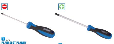
Screwdrivers manufactured from chrome vanadium steel with a satin chrome plated finish and a magnetised tip. The screwdriver is fitted with a bi-material soft grip handle providing user comfort, even when used for prolonged periods. The handles have a hanging hole, which can be used to place a 'T' bar through when extra torque is required. Display packed.
