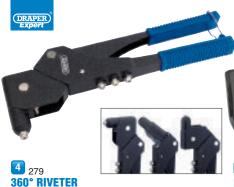
**Expert Quality**, aluminium head and body. Supplied with four nozzles to accept 2.4 3.2, 4.0 and 4.8mm aluminium rivets. Steel handle clip acts as nozzle change wrench. Display packed.
