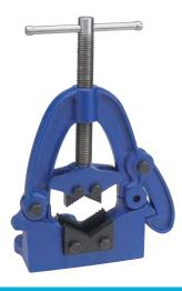
Ideal for repetitive clamping tasks on pipework. Can be fitted to a bench or a stand. The hinged top section allows rapid access to the job, whilst the self locking frame is reversible for right or left-handed operation. The steel tommy bar and mainscrew exert and maintain a powerful gripping force and the SG ductile iron frame is guaranteed unbreakable.
